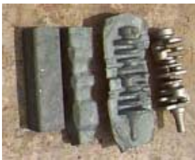
Left to right: (1) raw billet (2) rolled pre-formed billet (3) final forging (4) finished crankshaft
